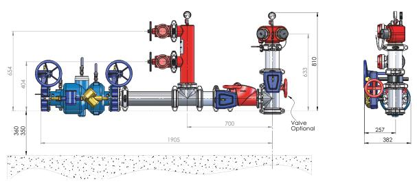
All Suction & Landing valves come fitted with Aluminium Forged alloy DIN Storz couplings as standard.
