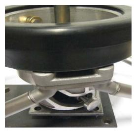
Assemble the two shafts for piston guide when applying pressure to the driving plate packet.
