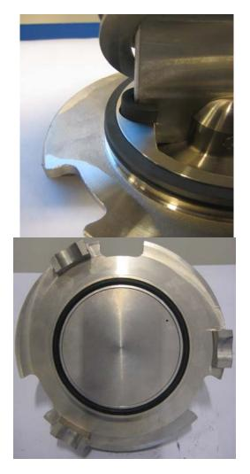
Change the Teflon® bushing (pos.13) to new ones on both sides.
