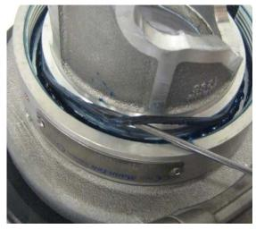
Change the O-ring (pos.24) from the groove in the coupling body.
