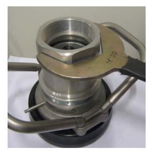
Place the swivel sleeve over the coupling body and screw in the swivel sleeve.
