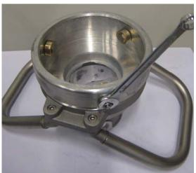
Change the three shafts (pos.18), locking nuts (pos.19) and rollers (pos.17) to new ones.
