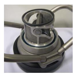
Change the Teflon® ring (pos.25) on the top of the coupling body.
