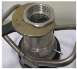
Mark the position of swivel sleeve against swivel ring with an Ø8 mm pin.
