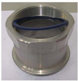
Place a new flat seal (pos.29) on the swivel sleeve. (Not needed when NPT-thread).
