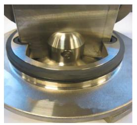
Change the O-ring (pos.8) and Teflon® ring (pos.9) on the driving plate back side. Use grease on O-ring.
