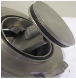
Change the O-ring (pos.3) on the piston. Use grease on the new O-ring. Make sure that the O-ring doesn't get twisted when mounting.
