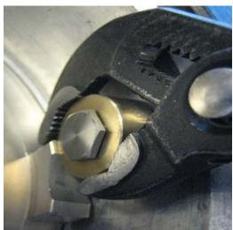
Turn the driving plate to the position where the recess ends up under the rollers under pressure to the driving plate packet.
