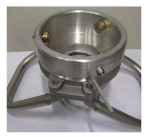
If necessary change O-ring (pos.21) for dust -protection. Use grease on the new O-ring.
