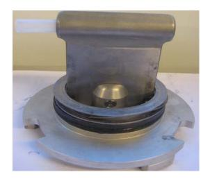
Change the Teflon® bushing (pos.16) to new ones on both sides.
