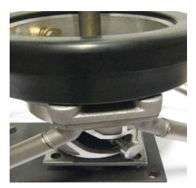
Remove the two shafts for piston guide, by applying pressure to the driving plate packet so that it moves down 2 mm. So that the driving plate packet is released from the rollers.
