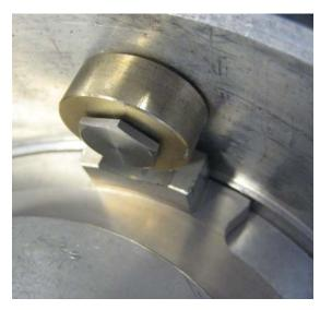
Press down and turn the driving plate to the position where the driving plate heels are placed under the rollers.
