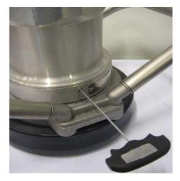
Use Loctite® 243 and screw the lock screw into the swivel ring without any force! Risk to deform the ball bearing!
