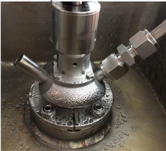
An aseptic valve uses a sealing around the stem to secure the inside of the valve body hermetically to the environment and avoid the so called "lift effect", which is created through the stem travel and thus can "pull" foreign bodies from the environment into the process, which may lead to contamination.
