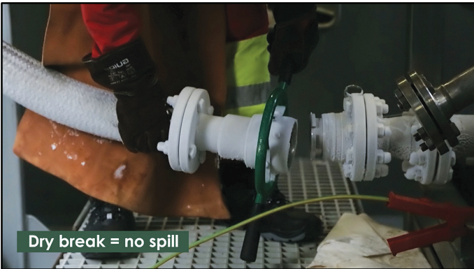
Disconnecting 3" Cryogenic Hose
